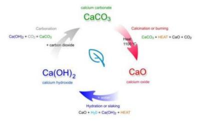
Figure 4 Cycle of Calcium carbonate-Calcium oxide-Calcium hydroxide.
